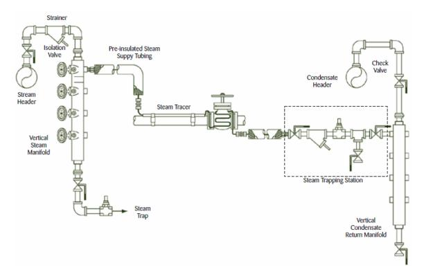
Typical Steam Tracing System (Figure Source: Thermon)
