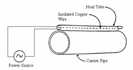
When the system is powered by high voltage (3 to 5kV), heat output occurs in both conductors. If the system is properly designed, 60 to 80% of heat output takes place in the steel tube, and only 20 to 40% in the inner conductor.
