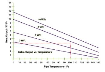
In this example, assume that the self-regulating cable is installed on plastic piping and over-wrapped with aluminum tape. The pipe maintenance temperature is assumed to be 100°F (38°C) and the calculation of overall heat loss is 4 W/ft. A vertical line is drawn
